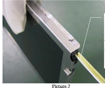
Push down the latch of the plastic frame (black) and insert the new Lamp Unit.
